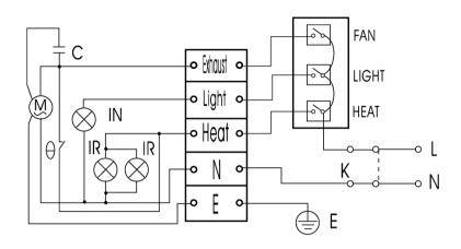
**NOTE**: This unit is fitted with a thermostat switch which will operate to automatically switch the exhaust fan on, in the event that the heat globes are left on, and the internal temperature of the unit exceeds 90°C.
