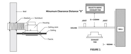
**CAUTION:** Ensure that the intended hole will have suitable room to locate the unit and that it will not interfere with joists or the ceiling structure. Joists, beams and rafters shall not be cut or notched to install the appliance.
